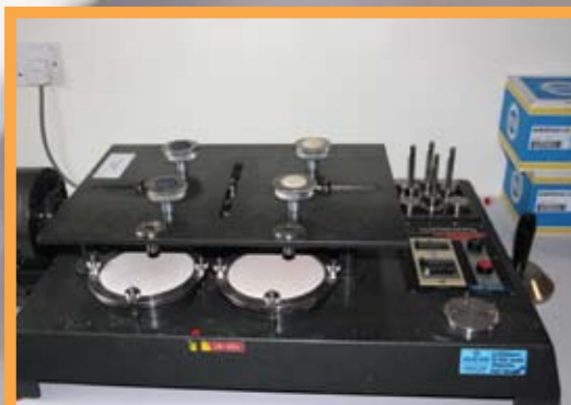
Martindale machine replicates abrasion by rock surfaces
